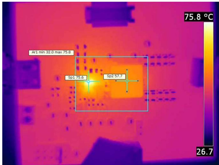
Figure 32. SP1: 75.6°C (TPS53515), SP2: 57.7 °C (Inductor)
