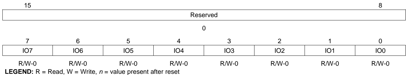
Figure 3-21. General-Purpose I/O Status Register (GPIOISR) [MMR Address 003Dh]
