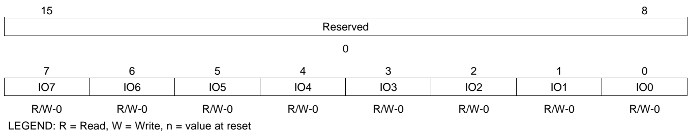
Figure 3-24. General-Purpose I/O Status Register (GPIOSR) [MMR Address 003Dh]
