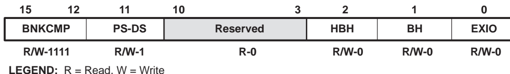
Figure 6. Bank-Switching Control Register (BSCR), MMR Address 0029h
