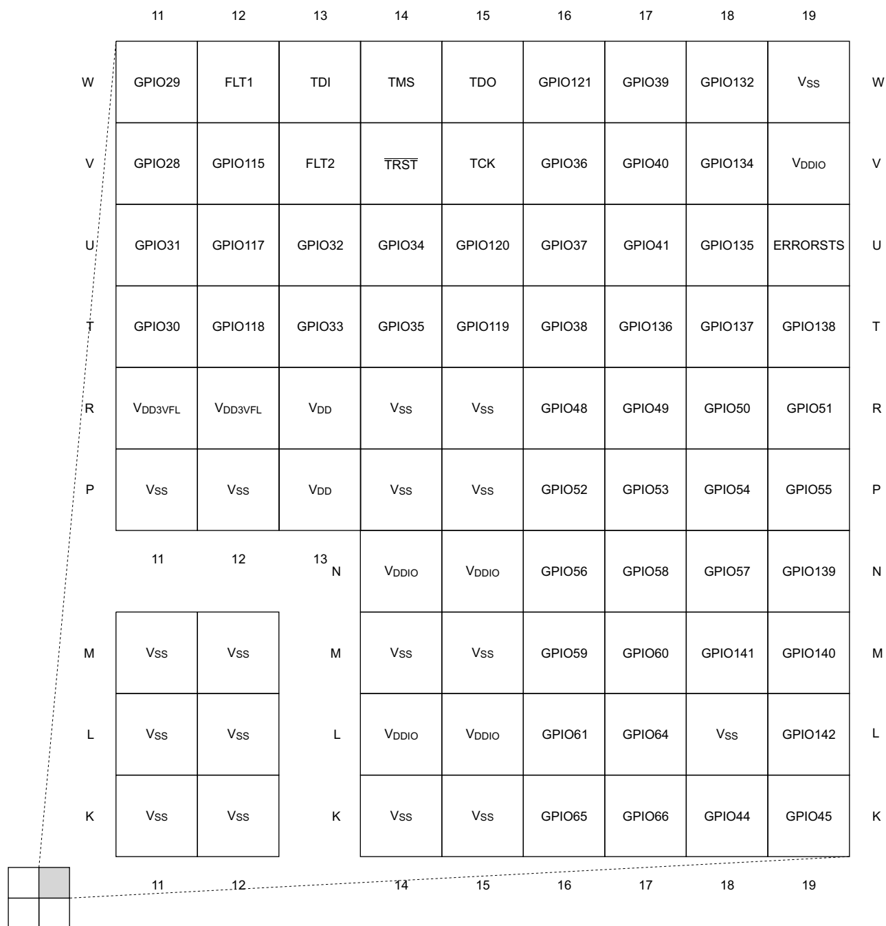
Figure 7-2. 337-Ball ZWT New Fine Pitch Ball Grid Array (Bottom View) – [Quadrant B]
