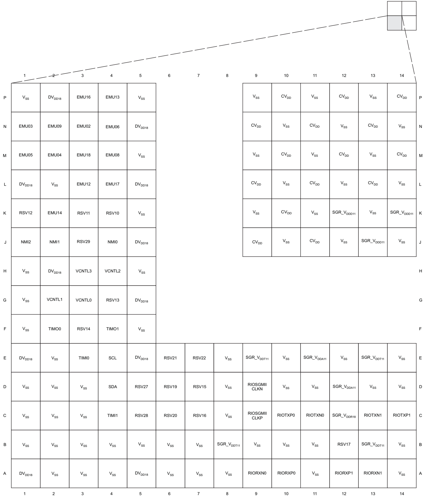
Figure 2-5. C6474 Pin Map (Bottom View) [Quadrant D]
