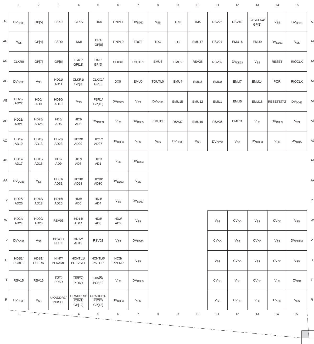
Figure 2-2. C6455 Pin Map (Bottom View) [Quadrant A]
