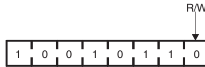
Figure 9. Software Reset Address
