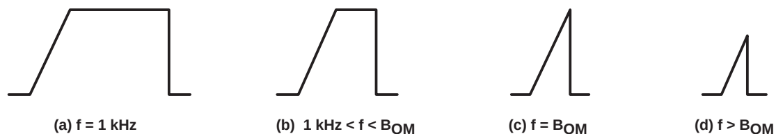
Figure 5. Full-Power-Response Output Signal
