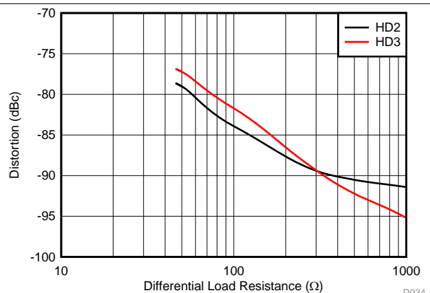
f = 10\text{ MHz} , see Figure 61 with V_{s+} = 3.0\text{ V} , V_{ocm} = 1.5\text{ V}
