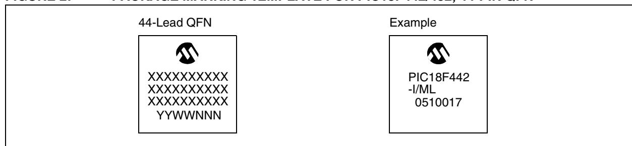
FIGURE 2: PACKAGE MARKING TEMPLATE FOR PIC18F442/452, 44-PIN QFN
