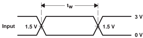
VOLTAGE WAVEFORMS PULSE DURATION
