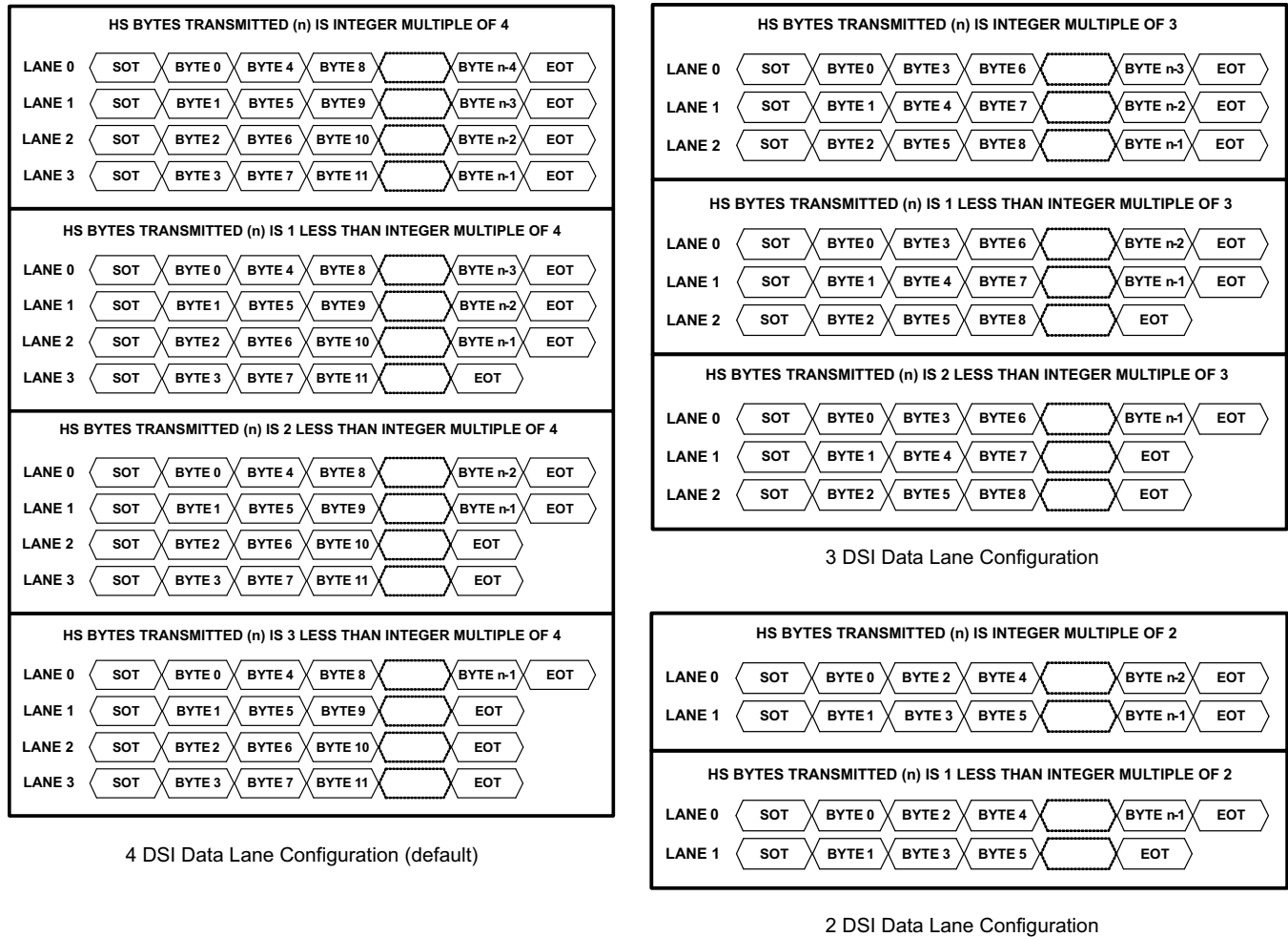
Figure 14. SN65DSI85-Q1 DSI Lane Merging Illustration
