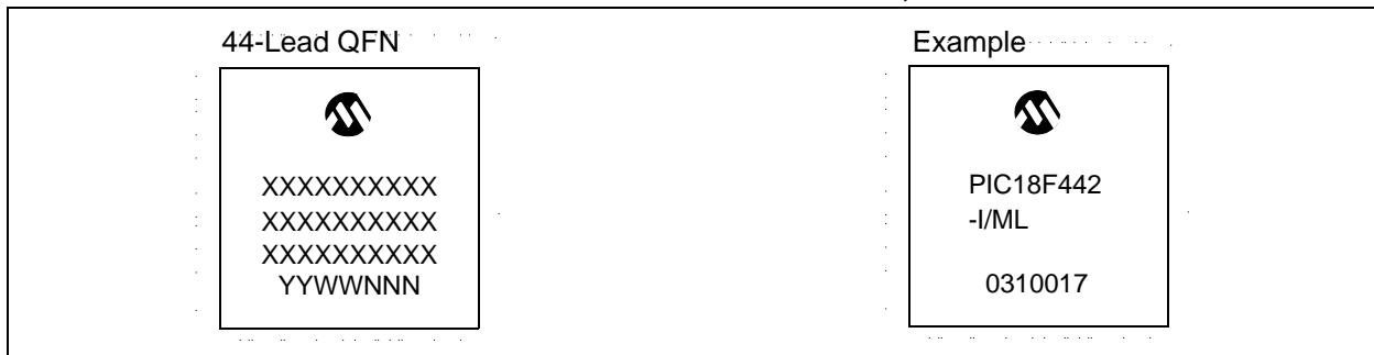
FIGURE 2: PACKAGE MARKING TEMPLATE FOR DEVICE#, 44-PIN QFN
