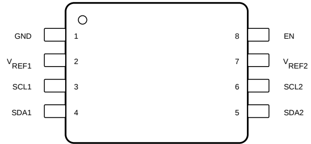
图 5-2. DCU Package 8-Pin VSSOP Top View
