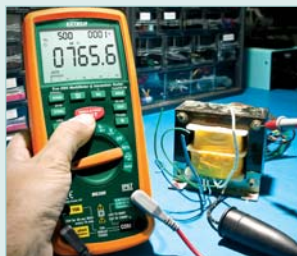
Measure the insulation resistance of transformer windings
