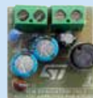
STEVAL-ISA178V1 5 V/200 mA buck-converter based on VIPer01
