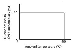
4. According to the ambient temperature, there are restrictions on power supply voltage and output load current for the CPU Units connected with the Expansion I/O Units (CP1W-8ER/16ER/20EDR1/32ER/40EDR). Use the PLC in the range of the power supply voltage and output load current as show below.
