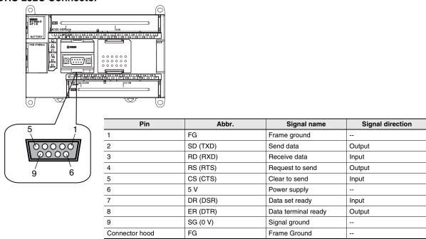
Note: Do not use the 5-V power from pin 6 of the RS-232C port for anything but CJ1W-CIF11 RS-422A Conversion Adapter, NT-AL001 RS-232C/RS-422A Conversion Adapter and NV3W-M□20L Programmable Terminal. The external device or the CPU Unit may be damaged.
