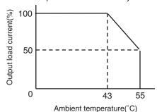
CP1W-32ER's maximum number of simultaneously ON output points is 24 (75%).
