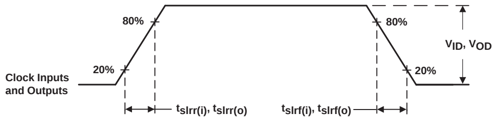
Figure 8. Input and Output Slew Rates
