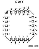
Note: Pin 1 is marked for orientation
