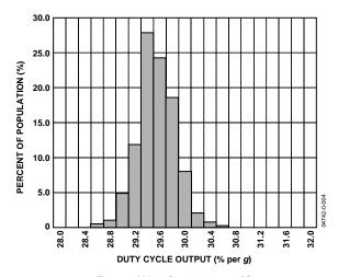
Figure 5. X Axis Sensitivity at 25°C
