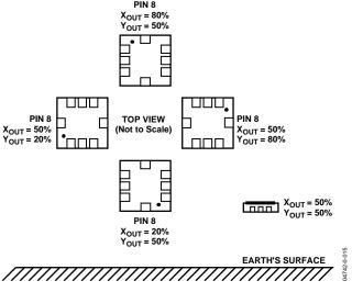
Figure 21. Output Response vs. Orientation
