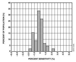
Figure 11. Z vs. X Cross-Axis Sensitivity
