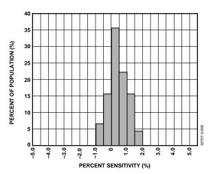
Figure 14. Z vs. Y Cross-Axis Sensitivity
