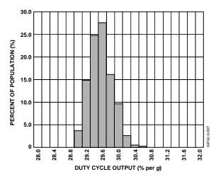
Figure 8. Y Axis Sensitivity at 25°C
