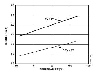
Figure 15. Supply Current vs. Temperature
