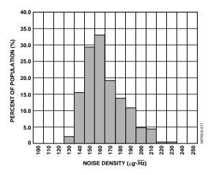
Figure 13. Y Axis Noise Density at 25°C
