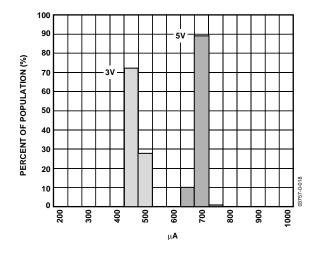
Figure 18. Supply Current at 25°C
