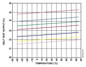
Figure 17. Self Test Response vs. Temperature
