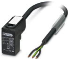
Sensor/Actuator cable, 3-position, PUR halogen-free, Black-gray RAL 7021, Free cable end, on C valve plug (8 mm), with 1 LED, connected with Z diode, Cable length: 3 m
